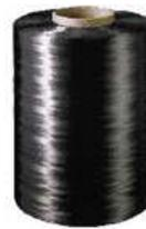
TORAYCA® carbon fiber is made by heat processing specialized acrylic yarn at temperatures between 1,000 to 3,000 degrees Celsius, and then winding tens of thousands of the resultant single yarns, which measure about a micron in diameter. It can also be combined with base materials such as resins to produce carbon fiber composite materials.
