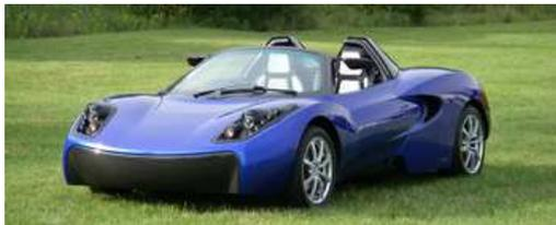
As Toray's flagship prototype, the TORAYCA® AR1 next-generation concept electric car embodies the Company's green innovation strategy. Toray used CFRP extensively in the car by applying its proprietary design and molding technologies, resulting in an extremely light vehicle weighing only 846 kilograms, about 66% lighter than a typical electric vehicle.
