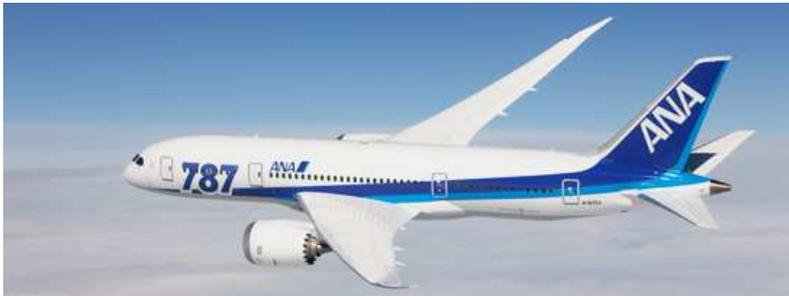
A totally carbon fuselage was achieved for the Boeing 787. CFRP was used as the primary structural material for the main wings, tail, and fuselage of the aircraft, and accounts for about 50% of the weight of the structural elements. (Photograph courtesy of All Nippon Airways Co., Ltd.)
