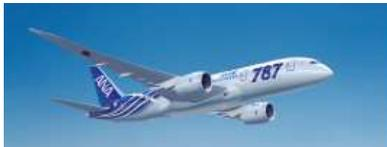
A totally carbon fuselage was achieved for the Boeing 787. CFRP was used as the primary structural material for the main wings, tail, and body of the aircraft, and accounts for about 50% of the weight of the structural elements.
