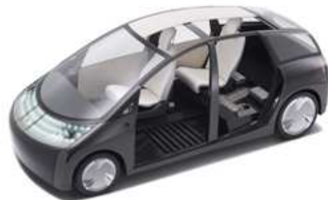
Toyota Motor Corporation's "1/X", an environmentally-friendly and safe concept car with CFRP used for the body frame
