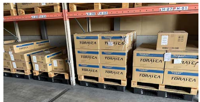
Pallets raised above the floor level (measure example)
