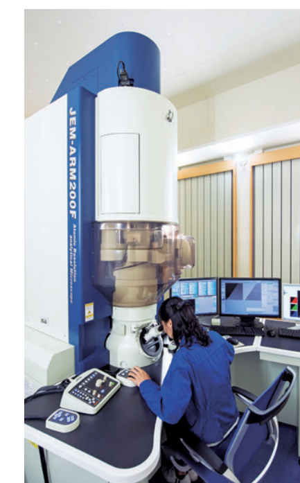
透過電子顕微鏡(TEM)観察 Transmission Electron Microscope (TEM) Observation
