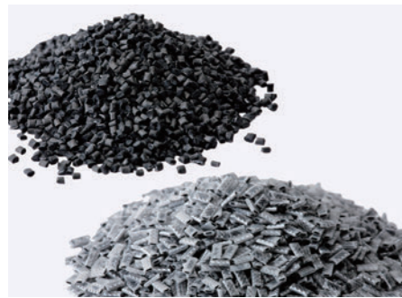
熱可塑性炭素繊維強化樹脂 Carbon Fiber Reinforced Thermo Plastics トレカ®樹脂 TORAYCA™ Resin
